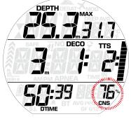
If the oxygen toxicity level reaches 75%, ascend to shallower depth to decrease oxygen loading and consider terminating the dive.
