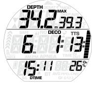
Pressing the button modifies the field in the bottom right corner in the following sequence:
