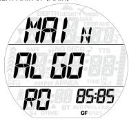
This is where you set the conservatism level of the ZH-L16C algorithm via gradient factors. We use Bühlmann's original values reduced by 15% as a starting point, and you can make the algorithm more conservative from there. There are four predefined sets of gradient factors with increasing conservatism from **R0 (85/85)** to **R3 (50/60)**. You can also enter the GF low and GF high values directly via the **CUStOM** setting. The default value is **R0 (85/85)**.
