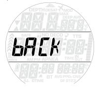
During the dive, press the button to access alternate information on the display and press and hold the button to activate the backlight.
