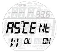
If the ascent rate exceeds 120% of the allowed value over a depth change of more than 20m/66ft, due to the potential of harmful bubble formation, Puck 4 locks the computer for 24 hours in order to prevent you from diving again. In this menu, you have the option to disable the locking up of the computer in the event of an uncontrolled ascent.
