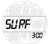
In this menu you can set the duration of the interval from the moment you reach the surface to when the dive computer closes the dive. During this interval you can submerge again and resume the dive. This menu allows you to change the default 3-minute interval to any value between 1 minute and 45 minutes.
