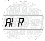
When selecting **NitROX**, you are taken to a submenu in which you can define the percentage of oxygen in the mixture  $(0_2\%)$  and the maximum value of oxygen partial pressure  $(ppO_2max)$  for up to three breathing mixes. The maximum possible value for the  $ppO_2max$  is 1.6bar. Most training agencies recommend not to exceed a value of 1.4bar.
