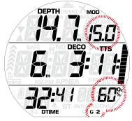
Press the button while this indication is blinking to initiate the gas switch: the oxygen percentage of G2 starts to blink in lieu of that of G1, and in the top right corner the MOD of G2 is displayed, also blinking.
