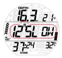
This persists until the ascent rate is reduced to below the pertinent limit. The limits are dependent on the current depth as follow:
