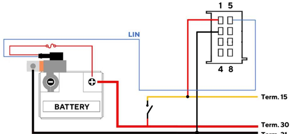
Remove the whole system from the negative pole of the battery and install the IBS on the pole instead.
